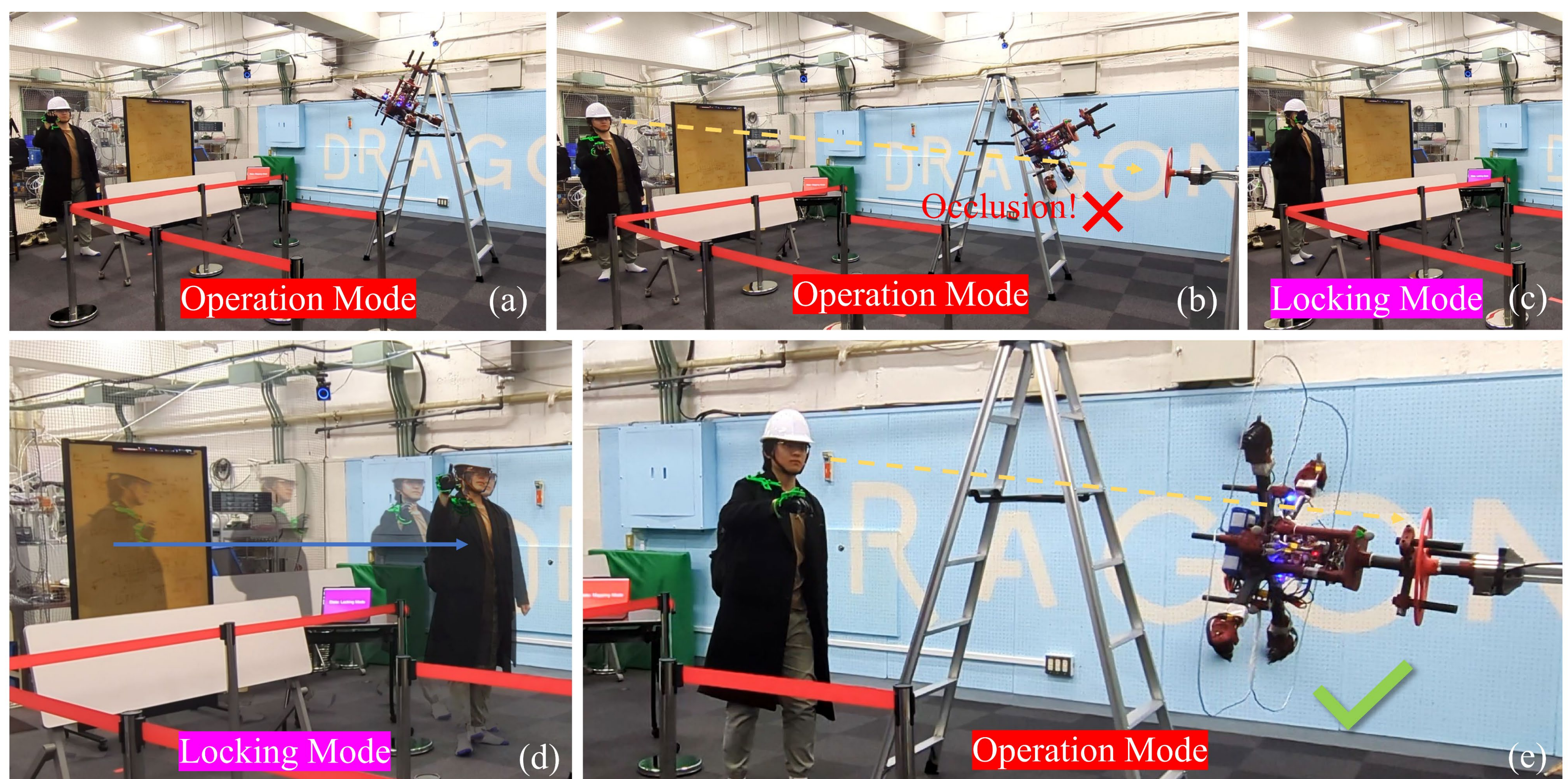
Fig. 8. Valve-Turning Scenarios: The operator switches to Operation Mode for precise manipulation, but the line of sight is blocked by the robot. To overcome this, they switch to Locking Mode , move to a different position, return to Operation Mode , and successfully complete the task.
