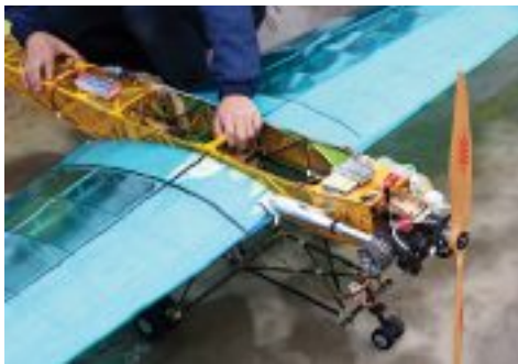
Beautifully-constructed craft with OS R21 Shimo buggy motor, scratch-built gearbox, tuned pipe and huge Sail prop (possibly Hebei Institute of Technology).
