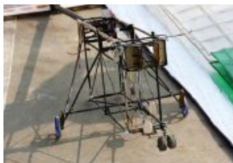
The same model's carbon bomb-rack, steerable nose wheel and rubber-sprung rear wheels.
