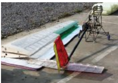
Another team's entry awaiting its engine – note all-carbon fuselage.
