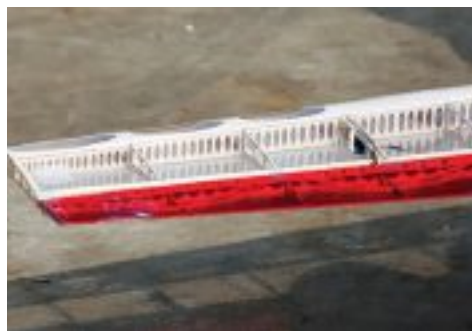
Maximum use of lightening holes in this beautifully designed & constructed wing.
