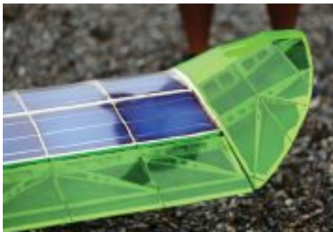
Lightweight Solar Aircraft challenge wing with blue solar panels and semi-geodetic rib work - (Maximum payload/empty weight) x flight duration = final score.
