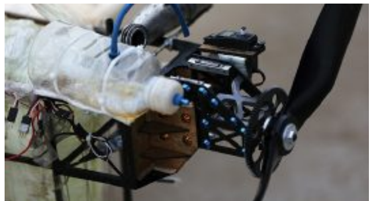
Engine removed showing carbon & alloy gearbox construction details.
