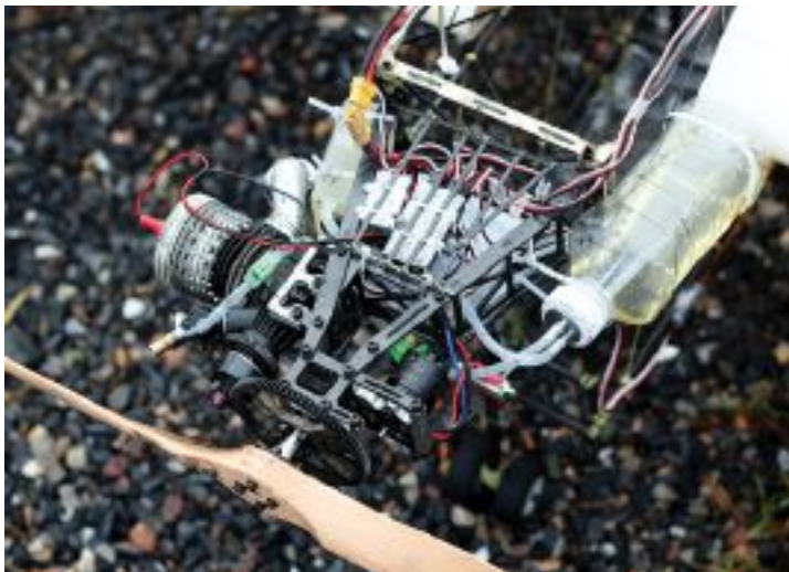
Another side-mounted OS R21 Shimo engine with complex gearbox construction, apparently incorporating an electric starter motor at lower right of photo.
