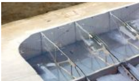
Some construction detail images follow – check out the lightweight construction (and sturdy L.E. box) here, using carbon, light transparent film – and lots of air!
